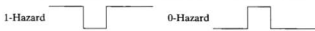
FIGURE 2-31 Waveforms produced by a circuit with (a) a static 1-hazard, and (b) a static 0-hazard.
