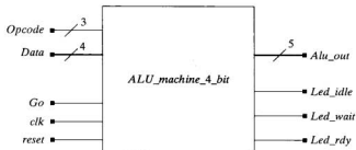
FIGURE P8-7a I/O ports for ALU_machine_4_bit .
